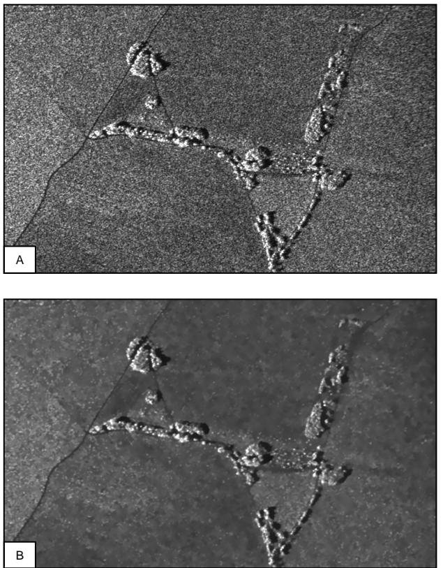
Figure 1. Speckle Suppression (A: original ; B: filtered)
