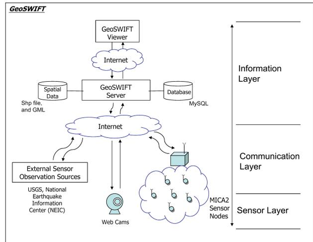
Figure 4. GeoSWIFT System Architecture Diagram
