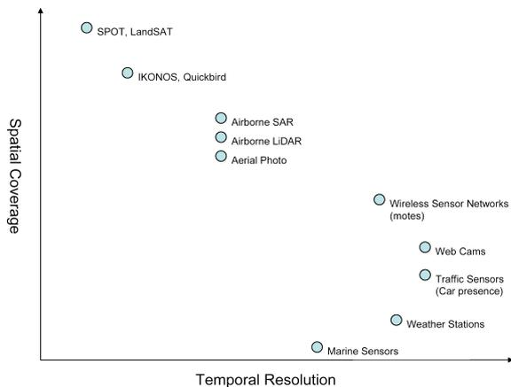
Figure 1. Sensor Web is an integrated sensing which has both large spatial coverage and high temporal resolution.
