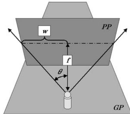
Figure 3-2. Relationship between focal length and field angle
