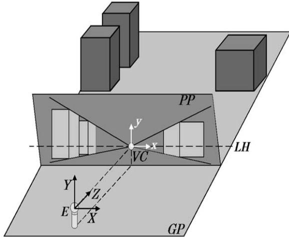
Figure 2. Schematic of perspective projection
