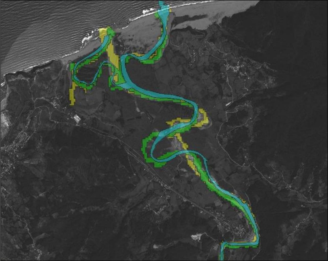
Figure 4. Superimposition of 2003 spot5 image onto the vectorized images relevant to the 1983, 1992, and 2000 for the changes in the river-bed and delta ( blue is 1983 segment, green is 1992 segment and yellow is 2000 segment).
