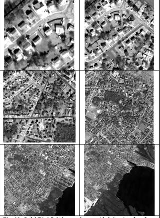
Fig. 10: QuickBird Sub-image shown with 0.6m, 1m, 2m, 5m, 10m and 15m ground resolution, same left upper corner
