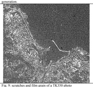
Film has the disadvantage of the photographic grain limiting the resolution and sometimes also disturbing the interpretation. In addition some of the handled photos have been disturbed by a high number of scratches (Figure 9). So for a TK350 photo
