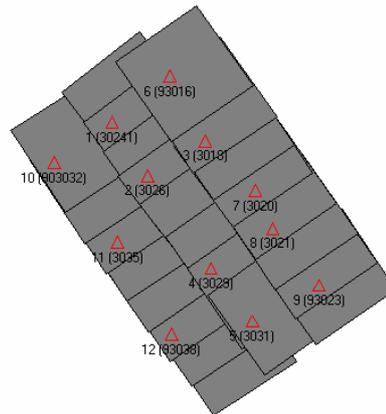
Figure 8. Block of 24 frame camera photographs taken at 880m flying height showing the distribution of ground control
