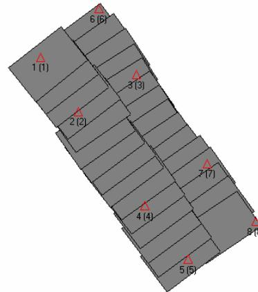
Figure 7. Block of 30 images taken at 760m flying height showing the distribution of ground control
