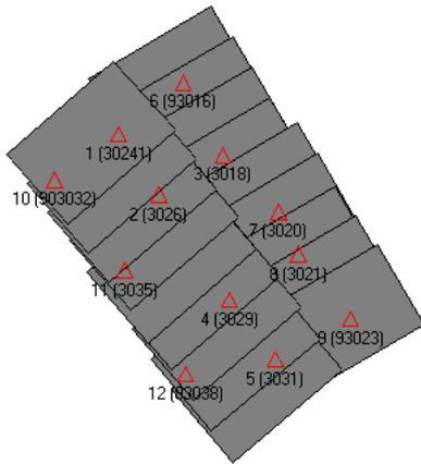
Figure 6. Block of 18 images taken at 1500m flying height showing the distribution of ground control
