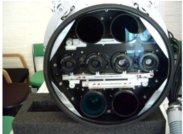
Figure 2. Multiple lens cones; 4 panchromatic across the centre and 4 larger colour cones (Copyright Simmons Aerofilms Ltd)
