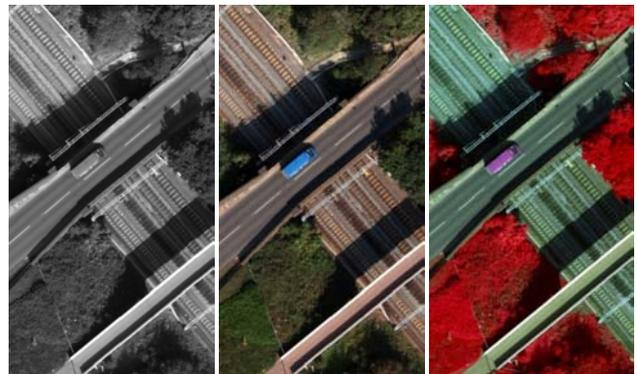
Figure 3. Panchromatic, colour and colour infrared images (Copyright Simmons Aerofilms Ltd)
