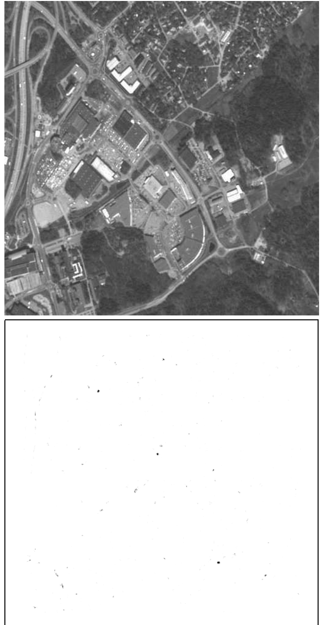
Figure 5: result of detection in a SPOT5 image ©CNES. The three darkest spots correspond to the three clearest roundabouts. So they can be detected with a well chosen threshold. However, there are other crossroads in this image which can be interpreted as roundabouts but they are not detected by the RAFA descriptor.
