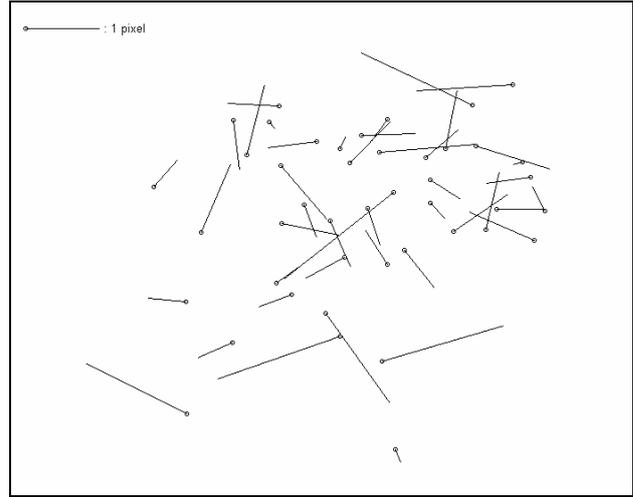
Fig. 2. Error vectors for the rigorous model using 44 GCPs.
