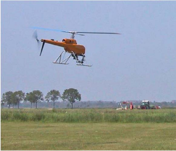
Figure 2. Helicopter UAV after Take-Off
