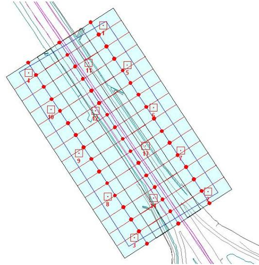
Figure 6. Typical Photogrammetric Flight Plan
