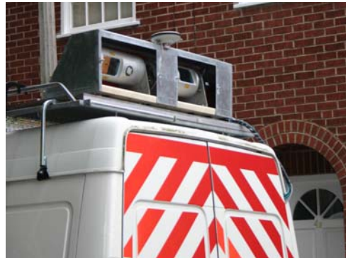
Figure 5. StreetMapper system with 2 laser scanners installed
