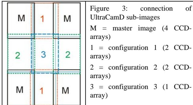
Figure 3: connection of UltraCamD sub-images
