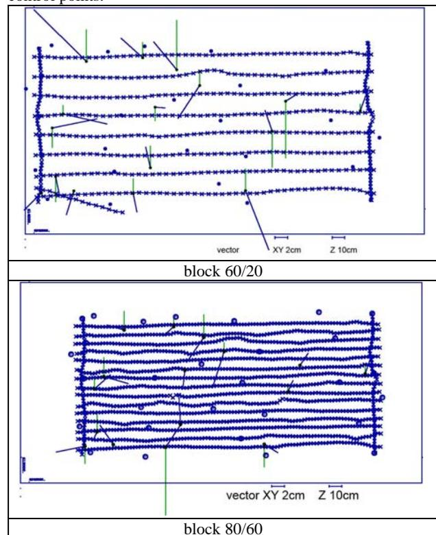
Figure 14: discrepancies at check points of block adjustment without self calibration
