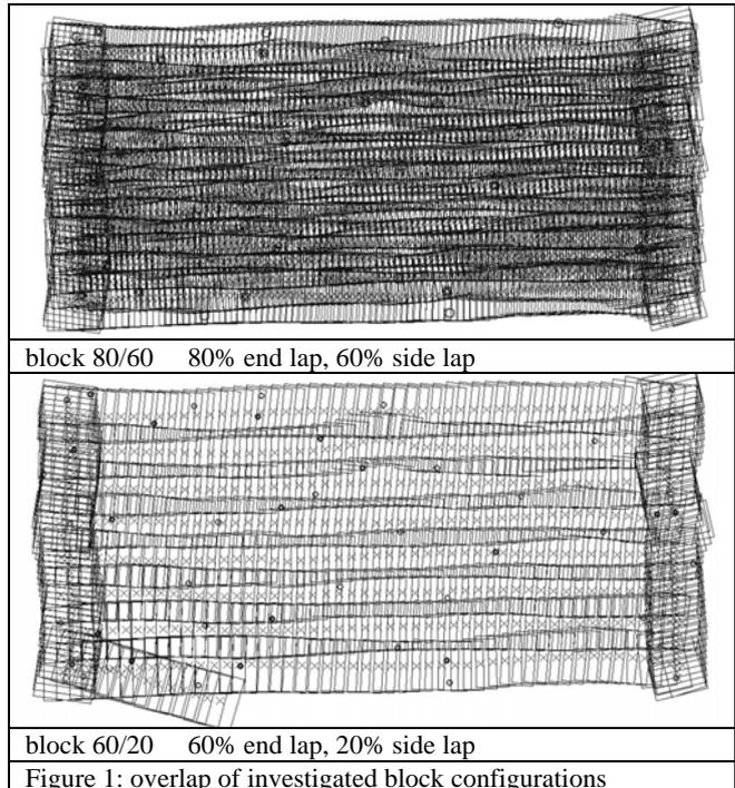
The blocks are stabilized by crossing flight lines at both ends, allowing a reduction of the number of control points. The partially varying side lap is caused by aircraft roll and not a deviation from the planned flight lines.
