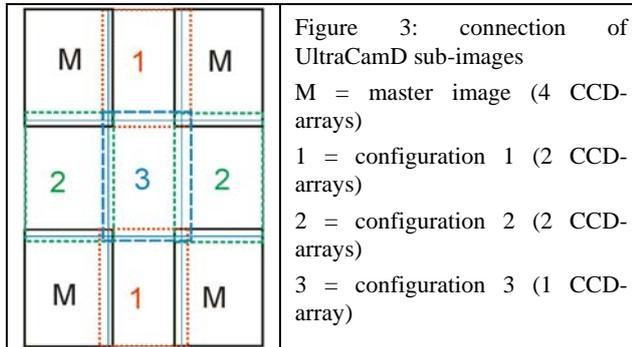
Figure 3: connection of UltraCamD sub-images
