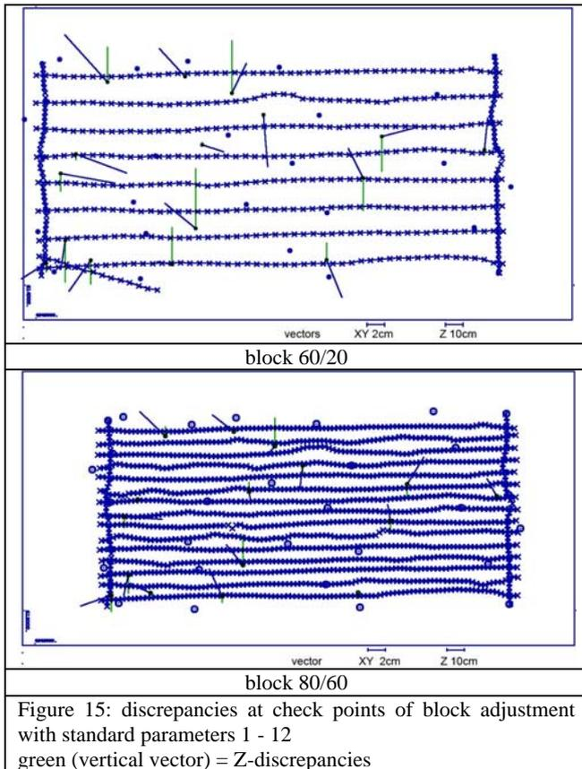
The block 80/60 with the strong overlap of the images is quite more stable like the block with the minimal overlap. Also from block adjustment with analogue photos the experience exists that with 60% side lap the distance of the control points can be extended.
