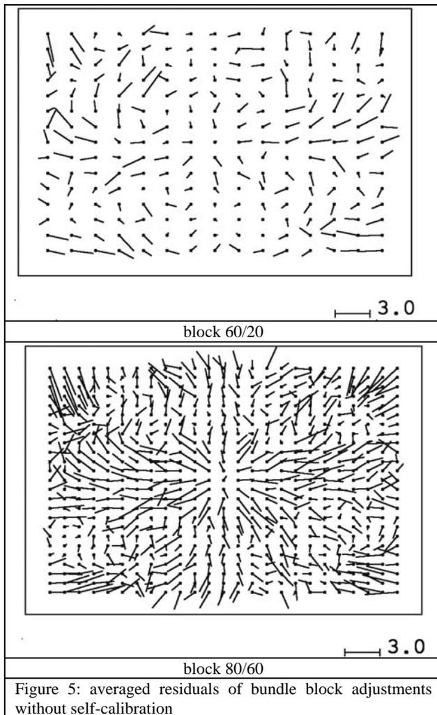
On the first view the averaged image residuals of the bundle block adjustments without self-calibration of both blocks seems to be different even if it is based on the same images. The dominating radial symmetric deformation of the block 80/60 cannot be seen so clear in the block 60/20. In block 80/60 the object points are measured in the average in 12.0 images while for block 60/20 we have only 4.4 images/point. That means in
