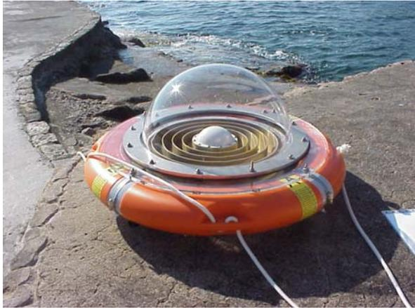
Figure 2: GPS Buoys used ain the calibration campaigns at l'Estartit area
