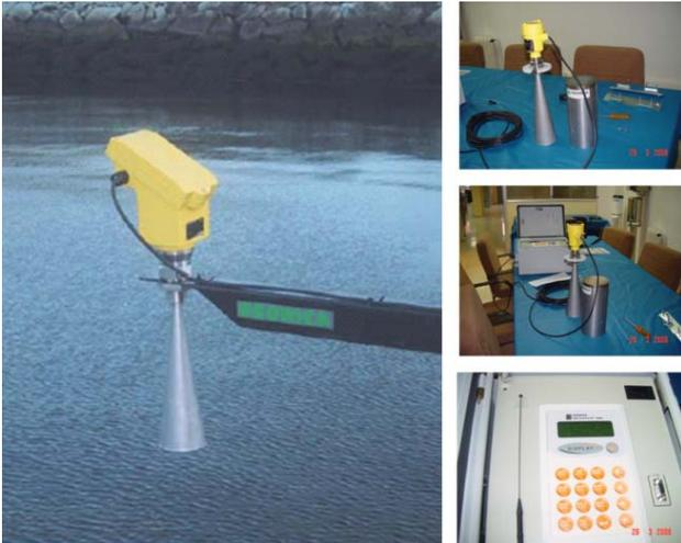
Figure 4: Radar tide gauge devices incorporating a GPS receiver for automatic clock synchronization ready to be installed at l'Estartit harbour. This modern installation will work in a parallel way to the classical floating gauge active since 1992. Images and deployments provided by Geonica sl, Earth Sciences.
