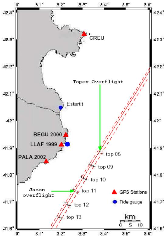
Figure 3: General distribution of the calibration area offshore Begur Cape indicating the surveying points on both the 1999-2000 and the 2002 campaigns. It is represented the nominal T/P ground track in the center and the parallel internal and the external ground tracks for the mapping of the sea surface.
