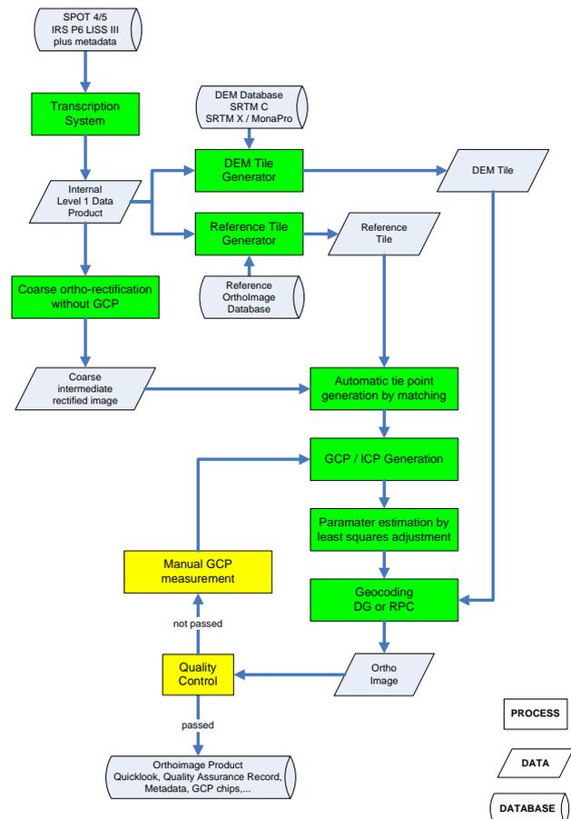
**Figure 1** Operational automatic processing chain for orthoimage production
