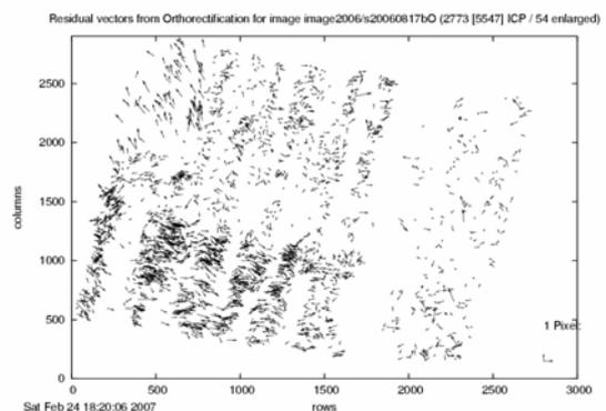
**Figure 3** Deviations in pixel - factor 54 enlarged - of automatically determined ICPs from the reference image versus image coordinates of the orthorectified scene (SPOT 4) after correction with GCPs ( $RMSE_x=12.6m$ ,  $RMSE_y=12.3m$ )
