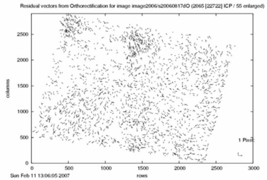
**Figure 2** Deviations in pixel - factor 55 enlarged - of automatically determined ICPs from the reference image versus image coordinates of the orthorectified scene (SPOT 4) after correction with GCPs ( $RMSE_x=12.4m$ ,  $RMSE_y=8.0m$ )
