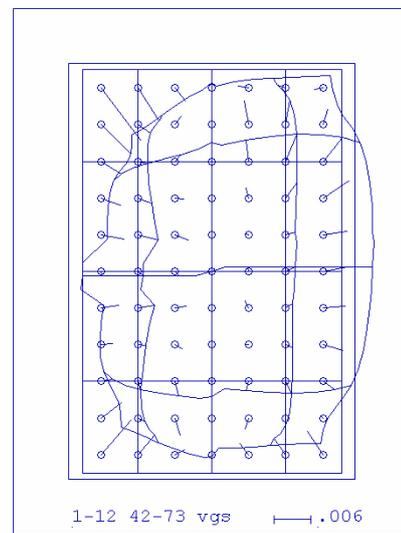
Figure 5 - Influence of UltraCamD additional parameters and BLUH standard parameters to image coordinates (units of the scale – mm)
