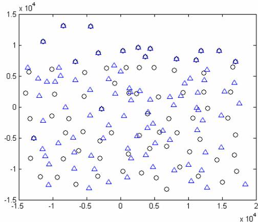
Figure 2 - Ground triangulation marks (triangles) and GPS determined ground points (circles)
