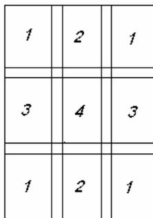
Figure 3 – Panchromatic mosaic sketch. 1 to 4: number of the source camera of the partial image.
