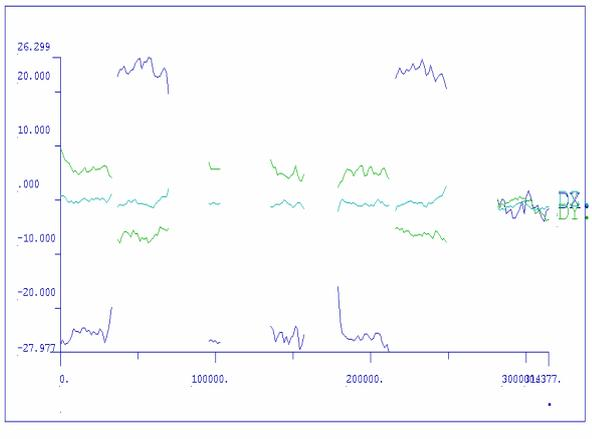
Figure 6 - Differences between AT-projection centers and GPS/IMU data (m)
