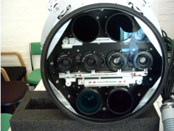
Figure 1. Multiple lens cones; 4 panchromatic across the centre and 4 larger colour cones (Copyright Simmons Aerofilms Ltd) (Smith et al., 2005)
