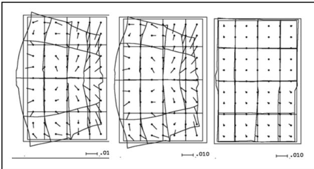
Figure 11: UltraCamD-block “DSK-Saar”: systematic image errors of flight campaign day1 (left) and day2 (center), difference of systematic image errors day1-day2 (right)
