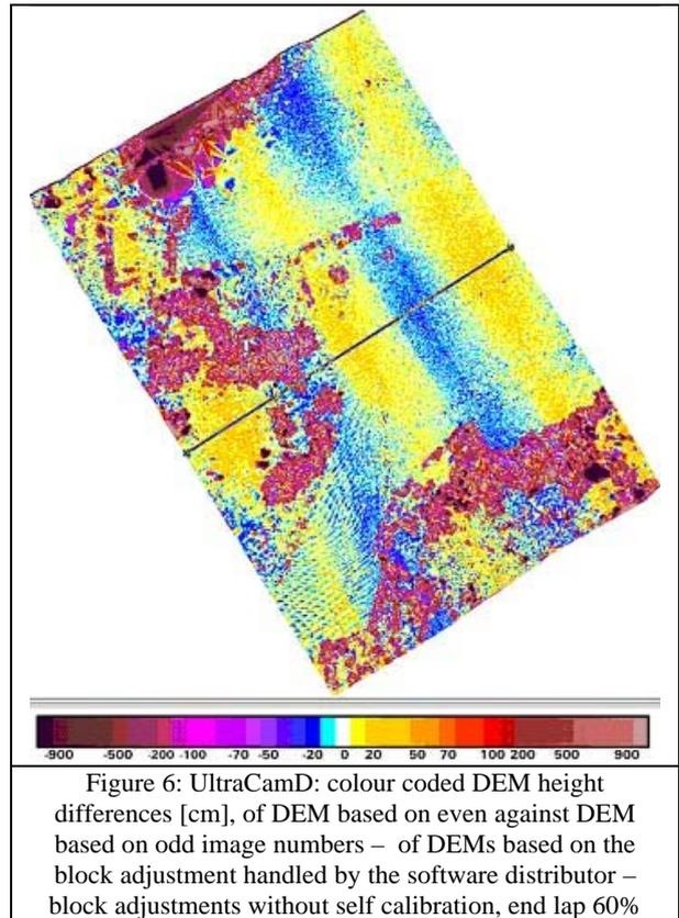
Figure 6: UltraCamD: colour coded DEM height differences [cm], of DEM based on even against DEM based on odd image numbers – of DEMs based on the block adjustment handled by the software distributor – block adjustments without self calibration, end lap 60%
