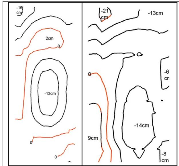
Figure 17: UltraCamD-block “DSK-Saar”: model deformation caused by systematic image errors based on additional parameters 1-12 (left) and 1-12, 42-73 (right); 9cm GSD, **end lap 49,5%**,  $h/b=2,9$ . Contour interval: 5cm
