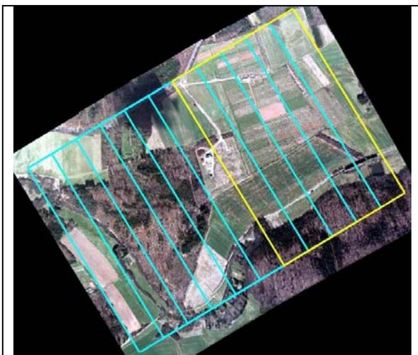
Figure 2: Block "DSK-Saar": orthophoto and stereo models with 80% end lap
