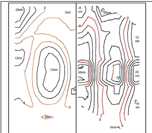
Figure 16: UltraCamD-block “DSK-Saar”: model deformation caused by systematic image errors based on additional parameters 1-12 (left) and 1-12, 42-73 (right); 9cm GSD, **end lap 66,3%**,  $h/b=4,4$ . Contour interval: 5cm
