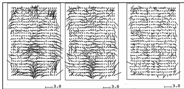
Figure 12: UltraCamD-block “Frederiksstad”, 17cm GSD, averaged residual without self calibration (left), parameters 1-12 (centre) and with parameters 1-12, 42-73 (right)
