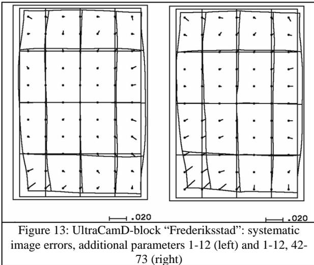
Like before a bundle adjustment with self calibration is required. Against a block adjustment with the general additional parameters 1-12 only a small improvement can be seen even if the remaining averaged residuals (fig. 12) indicate the requirement of the special UltraCamD parameters. The root mean square differences at the check point X- and Y-coordinates correspond to 0.31pixels and the 12.4cm in Z correspond to the hypothetical x-parallax of 0.20pixels for 60% end lap.
