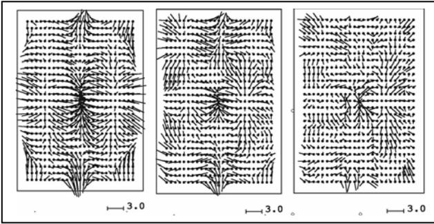
Figure 9: UltraCamD-block “DSK-Saar”, 9cm GSD, averaged residuals of block adjustment without self calibration (left), parameters 1-12 (center) and with parameters 1-12,42-73 (right)
