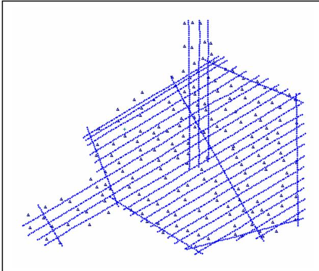
Figure 1: UltraCamD flight campaign "DSK-Saar", 2006: configuration of projection centers and ground control points
