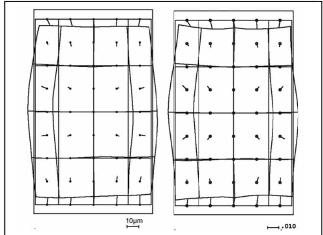
Figure 15: DMC-block "Frederiksstad": systematic image errors, additional parameters 1-12 (left) and 1-12, 30-41, 74-77 (right).
