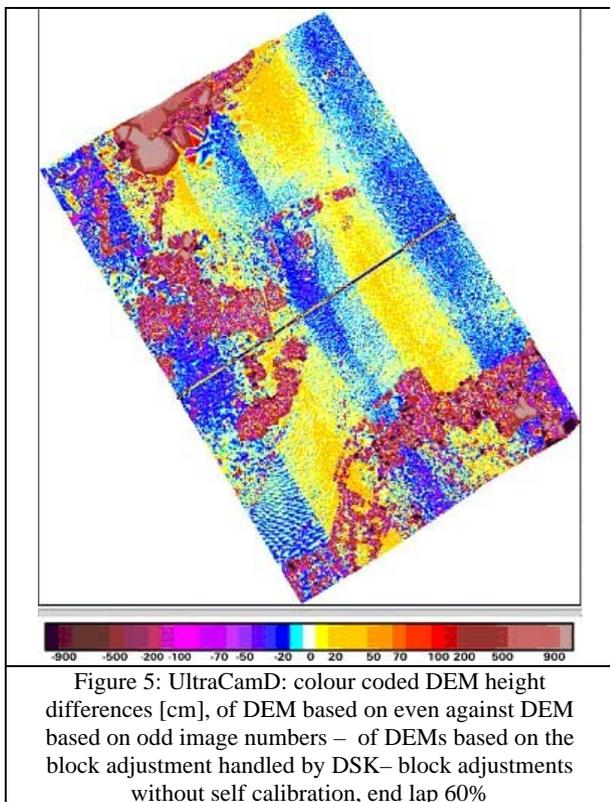
Figure 5: UltraCamD: colour coded DEM height differences [cm], of DEM based on even against DEM based on odd image numbers – of DEMs based on the block adjustment handled by DSK– block adjustments without self calibration, end lap 60%
