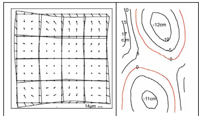
Figure 20: Analogue block “Frederiksstad”: systematic image errors (left) and model deformation (right) for analogue camera RMK TOP 15, photo scale 1:10600, **end lap 61%**, flying height above ground: 1620m
