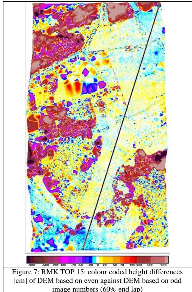
Figure 7: RMK TOP 15: colour coded height differences [cm] of DEM based on even against DEM based on odd image numbers (60% end lap)
