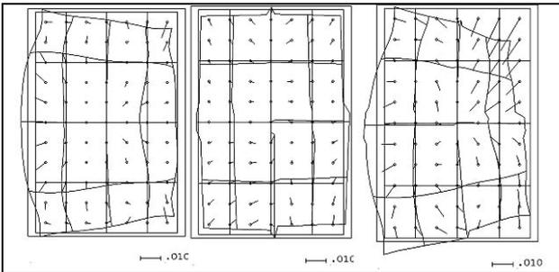
Figure 10: UltraCamD-block “DSK-Saar”: systematic image errors, additional parameters 1-12 (left), 42-73 (center), 1-12, 42-73 (right)
