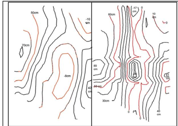
Figure 18: UltraCamD-block “DSK-Saar”: model deformation caused by systematic image errors based on additional parameters 1-12 (left) and 1-12, 42-73 (right); 9cm GSD, **end lap 84%**,  $h/b=9,3$ . Contour interval: 10cm
