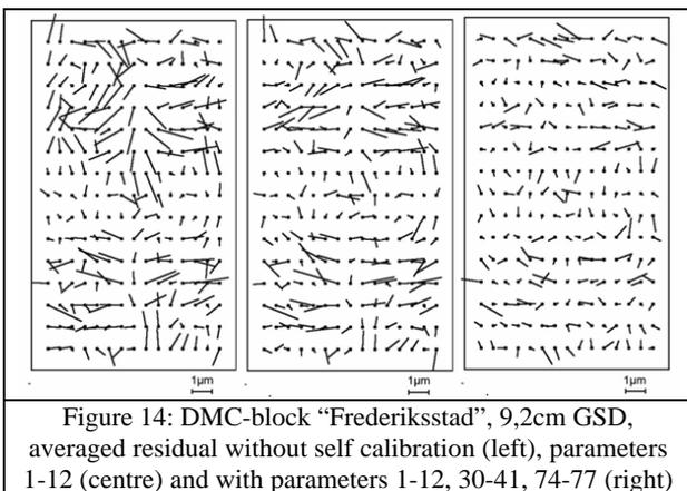
As expected, the results of the DMC block Frederiksstad show that self calibration is required and with the special additional DMC parameters the accuracy at the independent check points is more or less not improved. The same tendency exists for most of the handled DMC blocks (Jacobsen 2007). The adjustment
