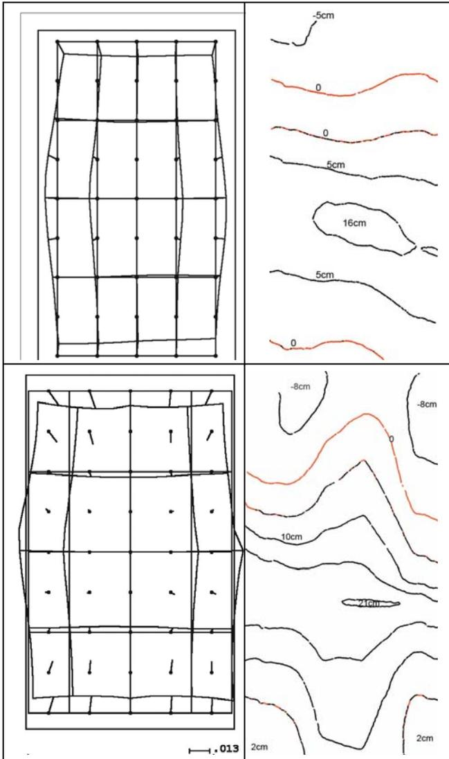
Figure 19: DMC-block “Frederiksstad”: systematic image errors and model deformation, 9,2 cm GSD, **end lap 63%**, parameters 1-12 (top), parameters 1-12, 30-41, 74-77 (bottom); 5cm-contour lines
