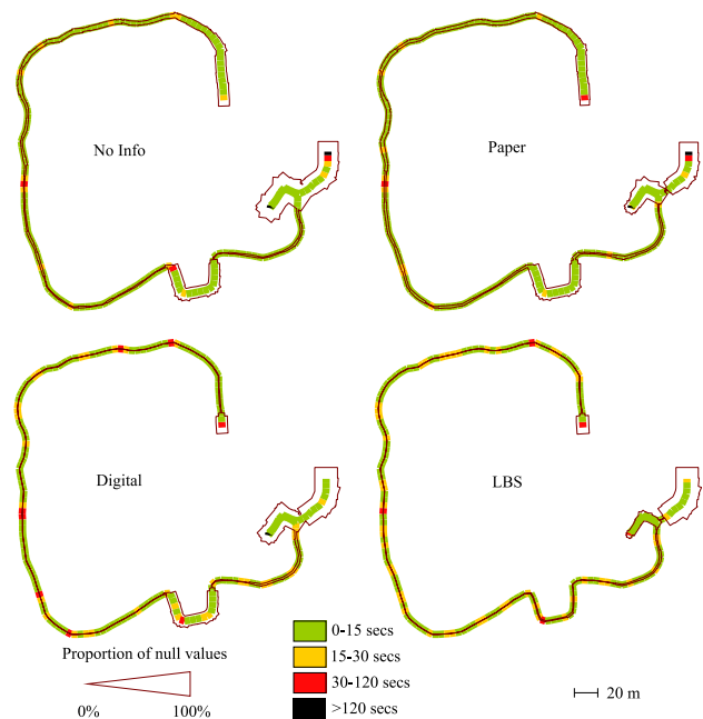
Figure 4. Average number of fixes per interval shown along the path for each information medium: a) No info; b) Paper booklet; c) Digital info and d) LBS.
