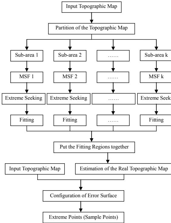
Figure 1. Flowchart for Spatial Sampling Scheme
