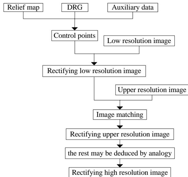
Figure 1 technique workflow
