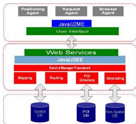
Figure2. Location Based Service Architecture
