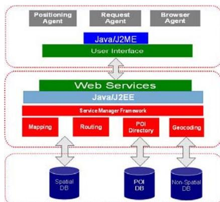
Figure2. Location Based Service Architecture
