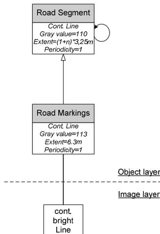
Fig.14: Road Model for the Minimal Configuration in ~5m/pel
