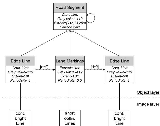
Fig.15: Road Model for the Maximal Configuration in ~5m/pel
