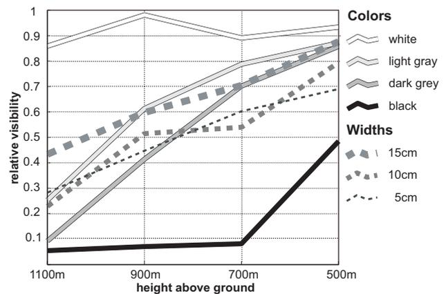
Figure 4: Height dependency of first returns statistics regarding the percentage of target hits in an area of slat width  $\pm$  geometric footprint size. The legend gives information about the different colors and widths. For the widths, all 4 colors have been put together.
