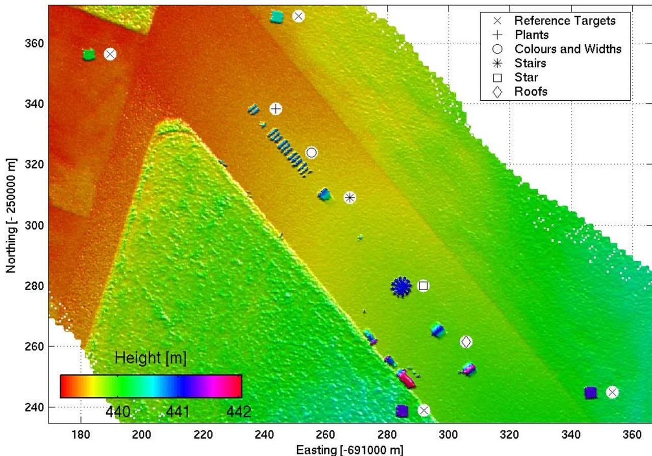
Figure 1: The Digital Surface Model (DSM) of our study site, an air strip. The positions of our reference targets are marked by white circles with the respective marker being explained in the legend. The DSM is from one of the 500 m above ground flights. The stair and the roof targets are not discussed in this paper due to the constraints in paper length.
