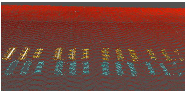
Figure 2: Slats with four different colors, white, light grey, dark grey and black (from left to right) and three different widths, 15, 10 and 5 cm (from left to right for each color). The length of the slats was three meter each. The lidar raw data from all 500 m AGL flights is superimposed. First echo data is colored orange to red, last echo data is colored cyan to magenta.
