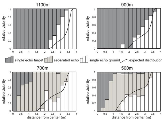
Figure 6: The ratio of echos from target to all echos from the center of the star to the outside. Color denotes the type of echo. The four panels are four different flying heights. For 500 m, all four flights have been put together.
