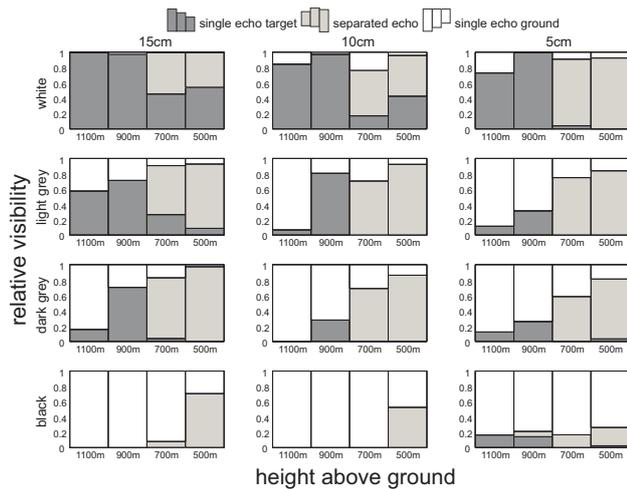
Figure 5: The percentage of target hits for the different colors (top to bottom) and different widths (left to right). The different colors denote different echo cases. White are ground echos (only single echos), light grey are separated echos (first always on target) and dark grey are single echos off the target. The different flying heights are labeled at the bottom of each plot.
