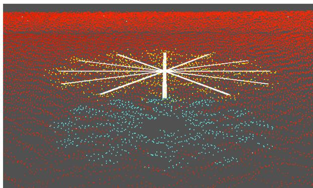
Figure 3: The *star* target. 12 white painted slats with a width of 5 cm were setup forming a star with a diameter of 6 meters and a height above ground of 1.5 m. The lidar raw data from all 500 m AGL flights is superimposed. First echo data is colored orange to red, last echo data is colored cyan to magenta.
