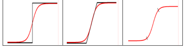
Figure 5: Calculation of structure points depending on edge type - step edge, ramp edge, curved edge (from left to right)
