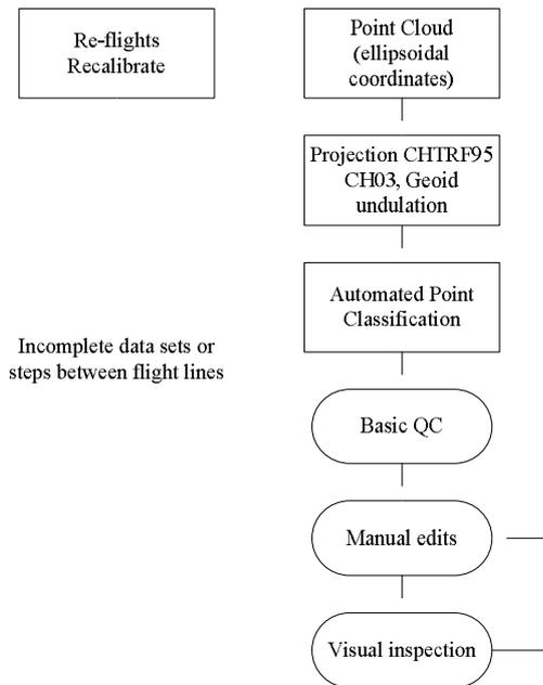
Figure 7. Flow chart of data post processing
