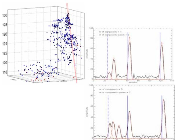
Figure 10. The additional points extracted from the waveforms (top left). The two lines indicate the travelling path for the waveforms to the right. The solid vertical lines show the position of the points extracted by the system. The dashed vertical lines show the position of the zero crossing of the second derivative for the first components. These positions correspond to a height value of 131.34 m (upper waveform) and 131.16 m (lower waveform).
