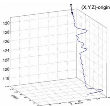
Figure 1. The waveform data was recorded in the mode 'last echo and earlier'. Each waveform contains 128 samples which correspond to about 19.2 meters. The first coordinate of the waveform (X,Y,Z-origin) and its direction vector were provided.
