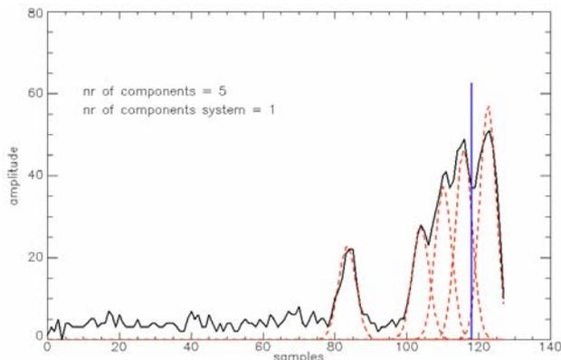
Figure 4. Waveform data (solid) and five estimated components (gray dashed),  $\mu_1=83.65$ ,  $\mu_2=103.89$ ,  $\mu_3=110.02$ ,  $\mu_4=115.99$ ,  $\mu_5=122.60$ . The vertical line symbolizes the position of the point extracted by the system.
