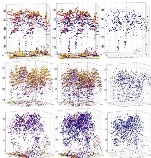
Figure 6. Point clouds for area 1-3, (15m x 15m). Pine trees (top row), spruce trees (middle row) and deciduous trees (bottom row). Extracted points by system (left column), from waveform data (middle column), and additional points extracted from waveform data (right column). The color indicates the intensity of the point.
