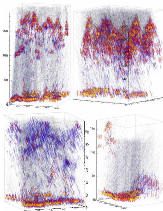
Figure 2. Volumes with waveform data. Area 1 (top left), area 2 (top right), area 3 (lower left), area 4 (lower right). The transparency is linear such that low values are more transparent. Voxel size: 0.15x0.15x0.15m<sup>3</sup>.
