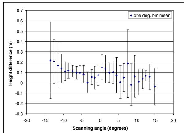
Figure 3. Calculated systematic and random errors for case (agricultural area) shown in Figure 2.
