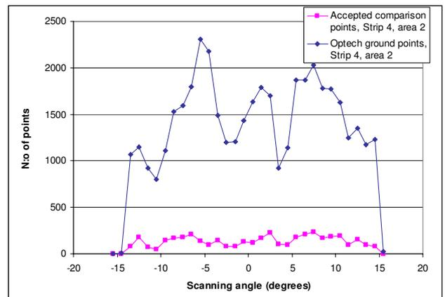
Figure 7. Amount of Optech ground points (above) and points used for verification (below).
