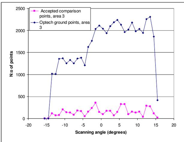
Figure 5. Amount of Optech ground points (above) and points used for verification (below). The drops at scanning angles more than 13 degrees (on the left) and more than 14 degrees (on the right) are caused by the loss of original data at these angles and it should not be taken into account.
