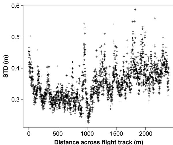
Figure 9. The standard deviation of pixels of the difference image of two laser based DTMs was calculated within all along track pixels and is shown as a function of distance in the across track direction.
