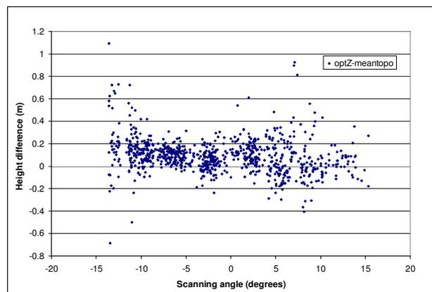
Figure 2. Height differences for agricultural field (strip 1, area 1). The amount of compared Optech points is 853.
