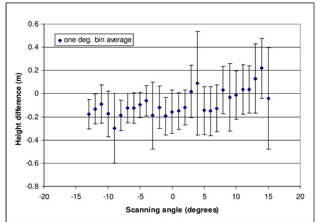
Figure 6. Calculated systematic and random errors for forest area. Strip 4, Area 2. 4084 verified points.
