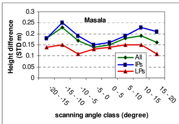
Figure 1. The elevation errors as a function of scanning angle for Masala test areas. All=all points, IPs=interpolated points, LPs=laser points.
