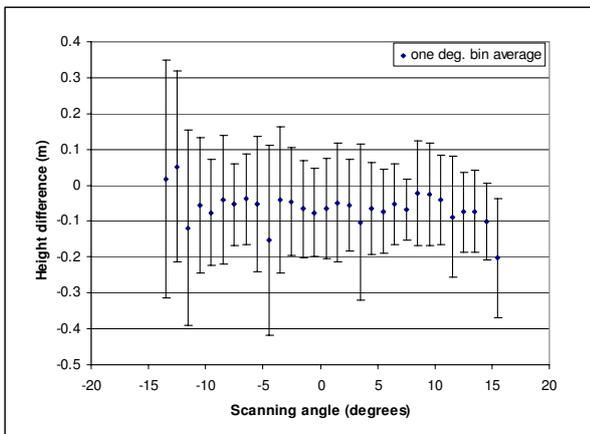
Figure 4. Calculated systematic and random errors for forest area. Strip 1, Area 3. 4683 verified points.
