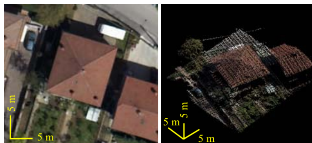
Figure 1. Left: orthophoto of one experimental area; right: view of laser points (colour by RGB from orthophoto).
