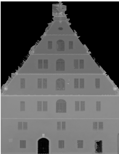
Figure 5. Top: Multiple georeferenced point clouds aligned with a virtual city model. Bottom: The LASERMAP of a single facade extracted from the data.
