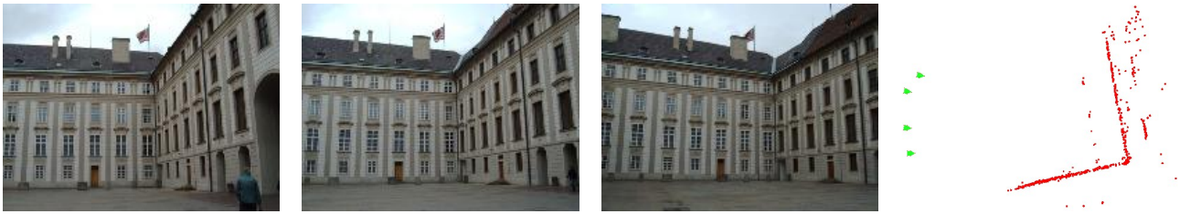
Figure 1: Three images of wide-baseline quadruple “Prague” and result after orientation and calibration (points in red, cameras as green pyramids; \sigma_0 = 0.24 pixels)
