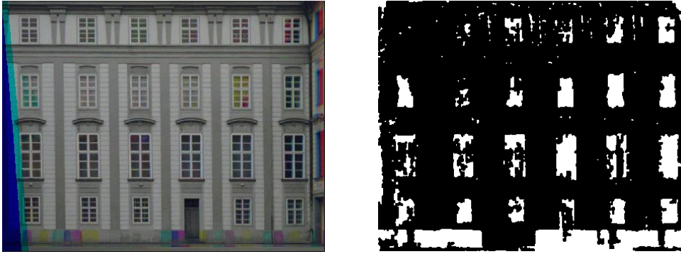
Figure 3: Three black-and-white images projected onto one of the façade planes mapped into the red, green, and blue image channel showing radiometric differences, but also deviations from the plane (left) and pixels on the plane (right)
