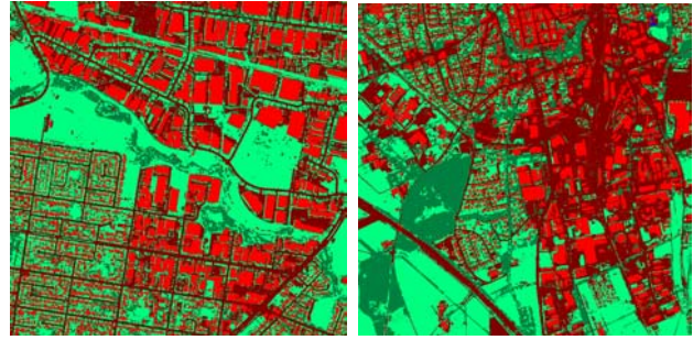
Figure 7. Results of the Dempster-Shafer classification after post-processing for Fairfield (left) and Memmingen (right). Light green: grass land. Brown: bare soil. Dark green: trees. Red: buildings.
