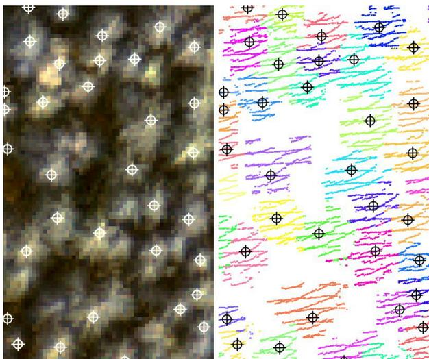
**Fig. 4:** Delineated trees in LiDAR point data: local maxima (left) and assigned laser point data (right).
