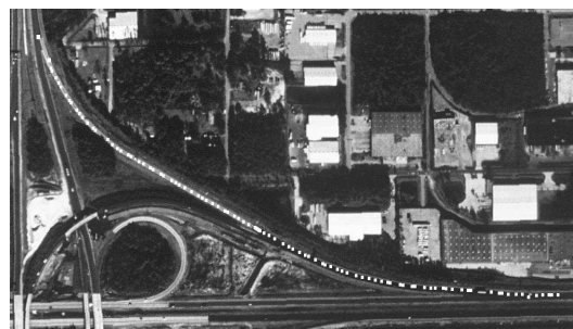
Figure 6: Road tracking from upper left corner to lower right corner. White dots are the detected road axis points, white line segment shows the location of human input.
