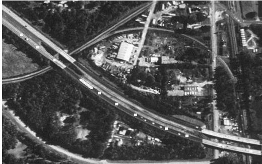
Figure 7: Road tracking from upper left corner to lower right corner. The number of human inputs is reduced by searching in multiple reference profile list, as described in the text.
