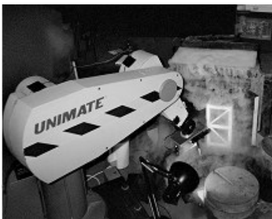
Figure 1. “Test sequence”-camera views a model oil-rig object in poor visibility.
