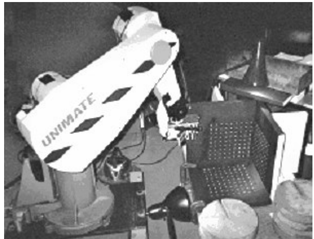
Figure 2. “Calibration sequence”-camera views calibration targets in good visibility.
