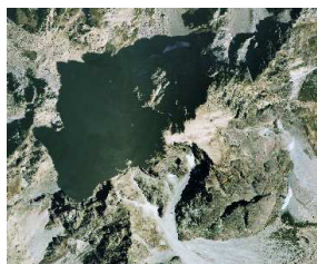
Figure 1: Example of large shadow area : the radiometry of pixels of a same class is different whether they lie in shadow or not
