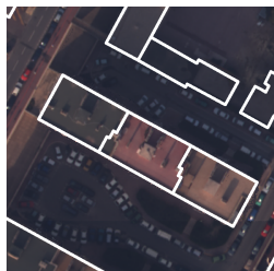
Figure 2: Semantic differences: one building can be split into 2 or more objects in the database.
