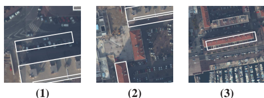
Figure 1: Update Problems. (1) : Destroyed buildings. (2) : New buildings. (3) : Planimetric inaccuracies.
