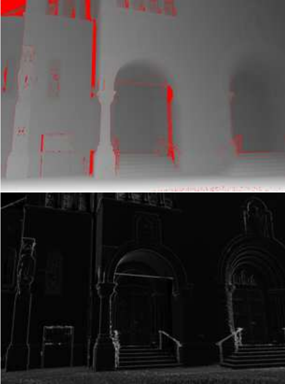
Figure 4: Mean \mathcal{D}_{\text{LIDAR}} (top) and variance \mathcal{D}_\sigma (bottom) of the depth with respect to one camera. Red pixels denote pixels for which the camera ray does not intersect the laser scan model.
