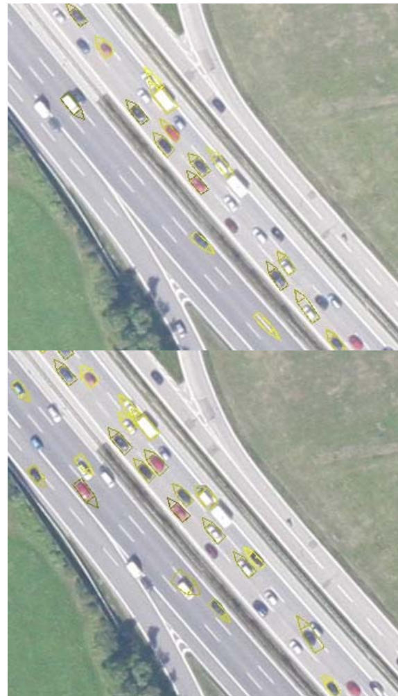
Fig 9. Zoom into the two images used for tests on the automatic vehicle detection. Rectangles mark automatic detections, triangles point into the travel direction.
