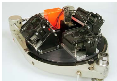
Fig 5. DLR 3K-camera system consisting of three Canon EOS 1Ds Mark II, integrated in a ZEISS aerial camera mount
