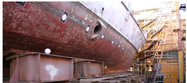
Figure 2. Waterline marked with black and white targets
