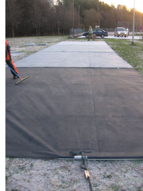
Figure 1. Four of the brightness calibration targets arranged for airborne laser measurement in Espoonlahti, Dec 2006. Each target is 5x5 m in size.
