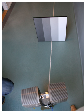
Figure 3. The FARO terrestrial laser scanner measuring a 4-step (12%, 25%, 50%, and 99%) Spectralon reflectance calibration plate (Labsphere Inc.).
