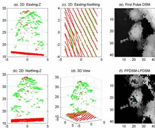
Figure 3. Points cloud corresponding to a deciduous tree, where a-f corresponds to cases in Fig. 1. Obviously, tree crown has been hit by the last pulse.
