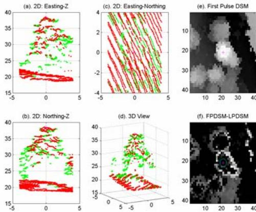
Figure 1. Points cloud and DSM corresponding to a coniferous tree. (a) Points cloud in vertical projection perpendicular to Northing, referred as Easting-Z. (b) Points cloud in vertical projection perpendicular to Easting, referred as Northing-Z. (c) Points cloud in horizontal projection, referred as Easting-Northing. (d) Points cloud in 3D space. (e) DSM based on first pulse laser data. (f) Difference between first and last pulse data.
