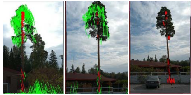
Figure 10. Using images for finding the trunk of the tree from the waveform data. The intersection of two perpendicular cross-sections finds potential echoes that have hit the trunk.
