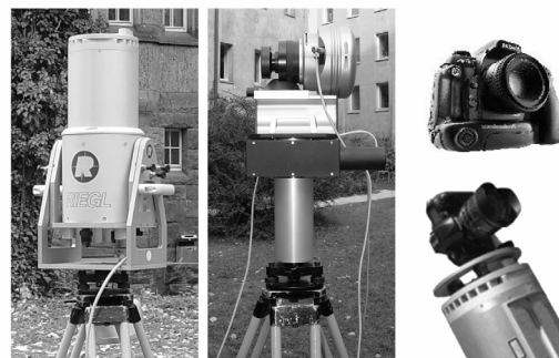
Figure 8. Combined devices (Riegl laser scanner LMS-Z420i, panoramic camera Eyscan M3, Kodak 14n, Nikon D100)
