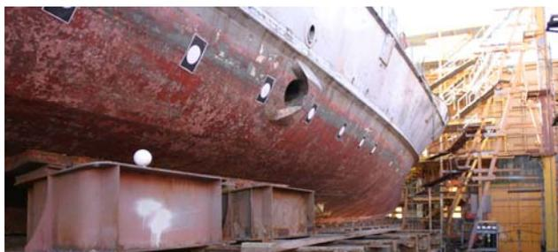
Figure 2. Waterline marked with black and white targets
