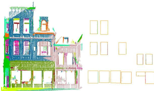
Figure 7. Another example showing extracted window is smaller than reality
