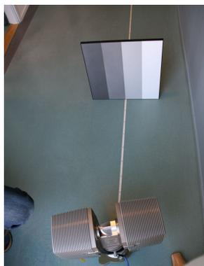
Figure 3. The FARO terrestrial laser scanner measuring a 4-step (12%, 25%, 50%, and 99%) Spectralon reflectance calibration plate (Labsphere Inc.).
