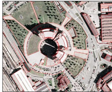
Figure 10. Orthophoto generated from a 20 cm DDSM.
