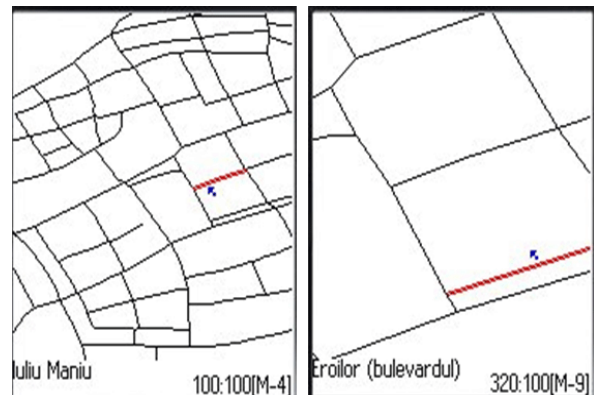
Figure 7. Street selection at low level (100%, sensitivity of 4 pixels) and higher level (320%, 9 pixels) of details.
