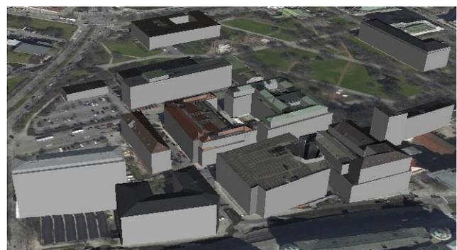
Figure 6. Stuttgart city around Applied Sciences University with roof texture is superimposed with Orthoimage and DTM
