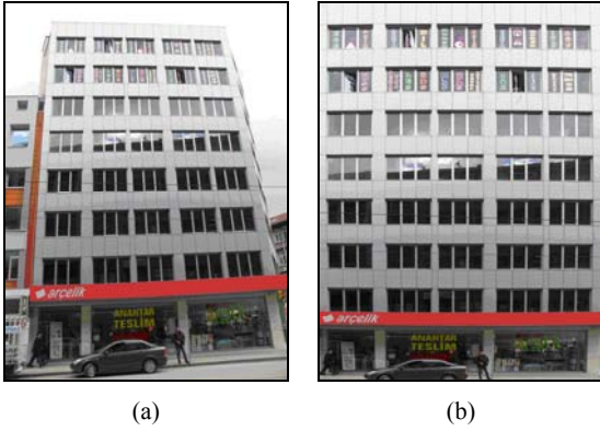
Figure 5: (a) Before and (b) after image rectification of an example façade image from the study area
