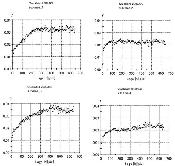
Figure 5. Comparison of semi-variograms of four sub areas divided in a similar way to Figure 2. The features of semi-variograms manifest the differences in both 'sill' and 'range' between high-density vegetated sub-areas and low-density ones.
