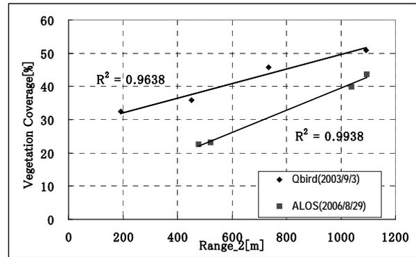
Figure 9. Correlation of vegetation coverage with longer 'range' value of semi-variogram of four sub-areas acquired by both 'Quickbird' and 'ALOS'. Unit of horizontal axis is converted to meters from their pixels. The threshold values of NDVI for calculation of vegetation coverage are 0.2 for 'Quickbird' and 0.12 for 'ALOS', respectively.
