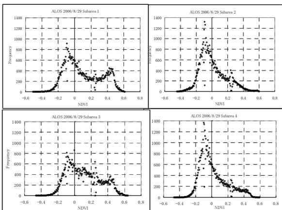
Figure 4. Comparison of histograms of NDVI values derived by 'ALOS AVNIR-II' sensors in four sub-areas. The distribution of NDVI values by 'ALOS' looks shifted to lower NDVI values by about 0.15.
