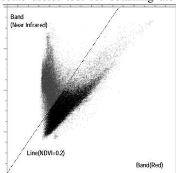
Figure 8. Scatter-plot of near infrared vs. visible red radiance values of 'Quickbird' sensor in a sub-area on September 3, 2003. A crossing line of plotted area indicates the threshold value of NDVI of 0.2 for calculation the percentage of vegetation coverage in the sub-area.
