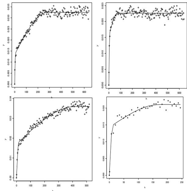
Figure 6. Fitted curves of semi-variograms to a combined spherical model with two 'sills' and 'ranges' in four sub-areas. Urban areas which contain less vegetation show a short value of semi-variogram's 'range' and fluctuating semi-variances around the 'sill' of semi-variograms as seen in sub-areas 'a2' and 'a4'.
