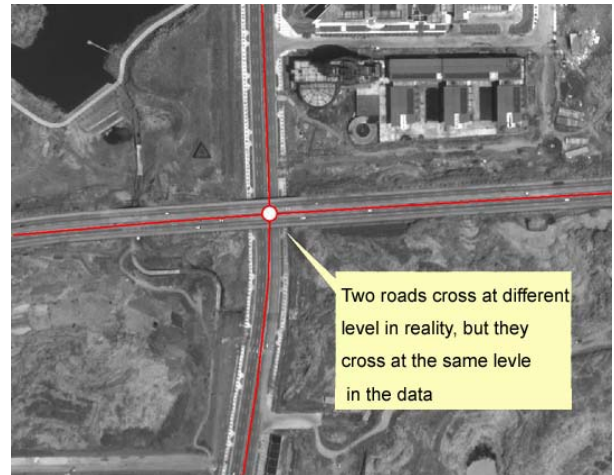
Figure 2. The representation of road in 1:50000 DLG
