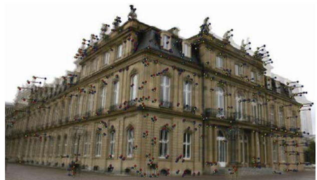
Figure 6: Overlaid image triplet with robust feature matches to determine the relative orientation.
