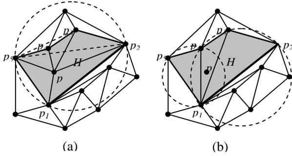
Figure 3. Deletion of non-constraint point  $p$
