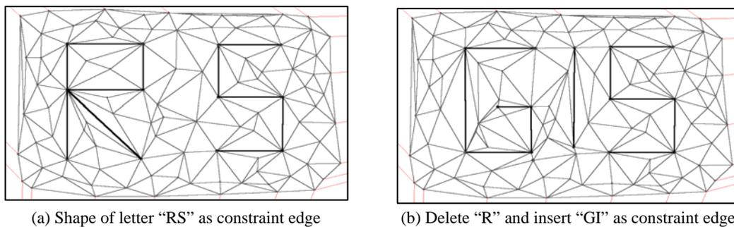
Figure 7. The shape reconstruction with dynamic deletion and insertion of letters in a CD-TIN
