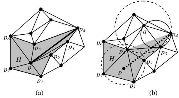
Figure 4. Deletion of constraint point  $p$
