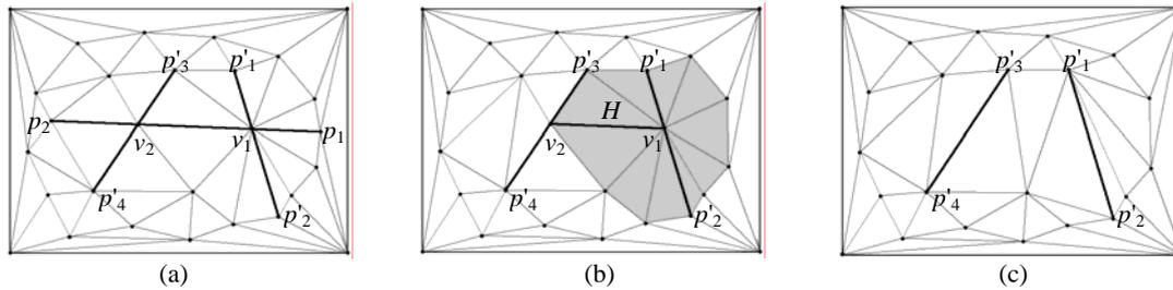
Figure 6. To delete constraint edges with virtual point
