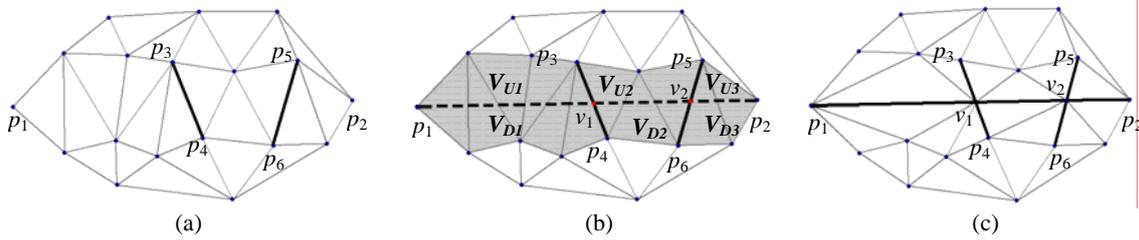
Figure 1. Virtual point insertion and re-triangulation.
